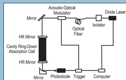
In the 1990s, Bergson explains, CRDS instruments were rare, bulky and expensive because these employed pulsed lasers. "What Lehmann determined was that you could use a small continuous wave laser the size of a contact lens, and not only achieve ring-downs but achieve better controlled ring-downs," she says. These lasers, a product of the telecom
